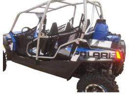
WHEN POLARIS DESIGNED THE FOUR SEAT RZR, THEY CREATED A ROLL BAR THAT INVADES THE AIRSPACE ABOVE THE REAR BED. PU-PRODUCTS RESPONDED BY CREATING A ONE INCH WIDE RZ-4 ADAPTER WHICH PROVIDES THE NEEDED SPACE TO ALLOW THE TRANSPORTATION OF OUR 5 GALLON JUGS.
